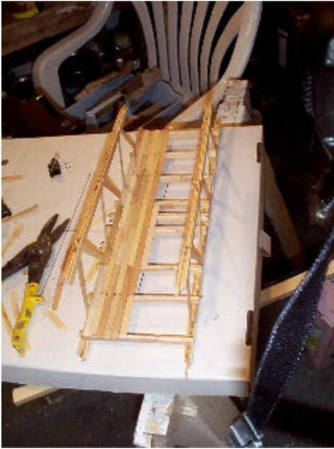
**Step 8:** Glue popsicle sticks to the deck beams to form the bridge deck and allow to dry. Unclamp the temporary bracing used to join the trusses together and glue the top braces across the top cord of the trusses. Remember to leave an opening in the center of the bridge to allow the testing apparatus to be placed on the bridge deck.
